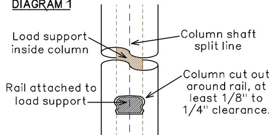
1. Measure the exact height at the location the column is to be installed. Be sure to include any draft angle your installation requires. The column must be trimmed 1/4" to 1/2" less than exact height.
