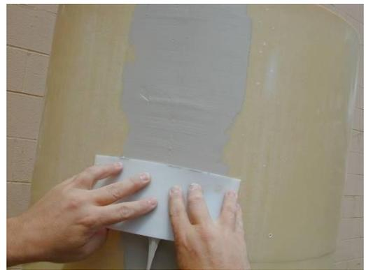
5) Smooth the body filler into a smooth radius using a thin sheet of plastic. You may have limited working time after catalyzing the body filler. Do not try to patch too large an area.
